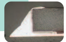
Thermal Cycling 200 cycles of -25 to +125°C, 20 mins dwell, 55 mins total cycle time
