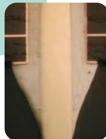
Thermal Cycling 200 cycles of -25 to +125°C, 20 mins dwell, 55 mins total cycle time
